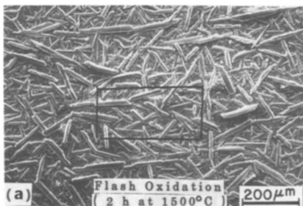
Figure 4 SEM micrographs showing the nature and morphology of the oxide scale after "flash oxidation" (2 h at 1500°C in air) of a SRBSN specimen.
